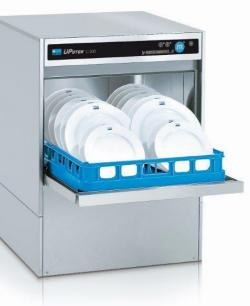
Entry height H 320 mm Dimensions H 845 mm, W 600 mm. D 600 mm Rack dimensions 500 x 500 mm Cvcle Times 120/180/240 secs Litres Per Cycle 3 L Power 240V 50Hz, 2.8 kW, 15 amp –Single Phase Water Hot - Max 60 Degrees
