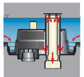
The original MEIKO eco-filter system filters the wash water in *UPster* machines, ensuring maximum hygiene and clean tank water.
